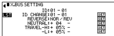
4. To assign 01-01 to the left elevator servo, scroll to the ID CHANGE field and set the main ID number to 03 and the sub ID number to 01. Scroll over to highlight SET and depress the scroll wheel. A notification will appear to indicate either a timeout (failure) or success. This lead's ID has now been set.
