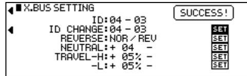
9. Once again, scroll back up to ID, and set the ID to 01-04 to program the lead labeled “4”. Failure to reset the ID field to the second lead’s default identification (01-04 versus 01-03, 01-02 or 01-01) will reprogram a previous lead.
