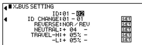
6. In the ID CHANGE field, set the main ID number to 04 and the sub ID number to 02. Scroll over to highlight SET and depress the scroll wheel to finalize settings. This lead's ID has now been set.
