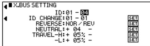
10. In the ID CHANGE field, enter a main ID number of 02 and a sub ID number of 04 this time, since there are two servos utilizing the aileron channel’s output signal. Scroll over to highlight SET and finalize.
