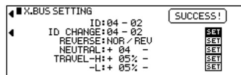
7. Scroll back up to ID, and set the ID to 01-03 to program the lead labeled “3”. Failure to reset the ID field to the second lead’s default identification (01-03 versus 01-02 or 01-01) will reprogram a previous lead.
