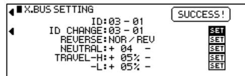
5. Scroll back up to ID, and set the ID to 01-02 to program the lead labeled “2”. Failure to reset the ID field to the second lead's default identification (01-02 versus 01-01) will reprogram the first lead.
