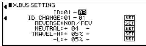
8. In the ID CHANGE field, enter a main ID number of 04 and a sub ID number of 03. Scroll over to highlight SET and depress the scroll wheel to finalize settings. This lead’s ID has now been set.
