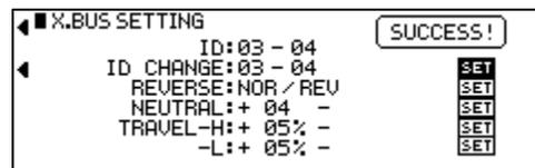
By now, you may have noticed, that if no ID changes were performed, the factory default for each of the leads would be set such that all four servos would move when the throttle (channel 01) stick was deflected. By changing the IDs and activating the SET command, we are able to now control two elevator servos, and two rudder servo out of the same harness. More importantly, we are able to control the physical lead into which the servo is plugged to customize wiring.
